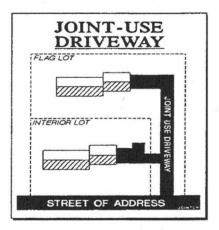
H. All driveways shall have a minimum of a six (6") inch crushed stone apron for a distance of twenty-five feet (25') from the paved edge of the street cartway and conform to the following detail:
