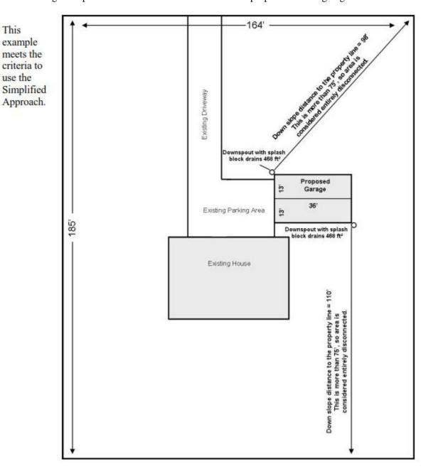
Step 1: Determine the area to each disconnected discharge. The area draining to each downspout is  $468 \text{ ft}^2$ . This is less than  $500 \text{ ft}^2$ , proceed to step 2.
